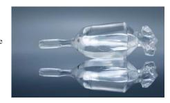
transmittance band width, large phase matching range, high damage threshold, and no tidal solution, and has become a research hotspot in frequency conversion devices. Due to Y can be replaced with most rare earth activated ions in any ratio, the crystal possesses both laser and nonlinear optical properties, thus becoming a laser self doubling crystal. The biggest advantage of YCOB crystal is its excellent nonlinear optical absorption and the ability to fabricate large aperture devices.
