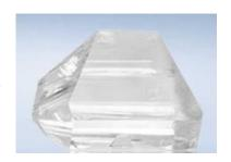
Using  $1.0~\mu$  M-band laser pumped non critical phase matching cut RTP nonlinear crystals and their isomorphs can achieve efficient 1.5- $1.6~\mu m$  band eye safe laser, has important applications in the field of nonlinear optical frequency conversion.
